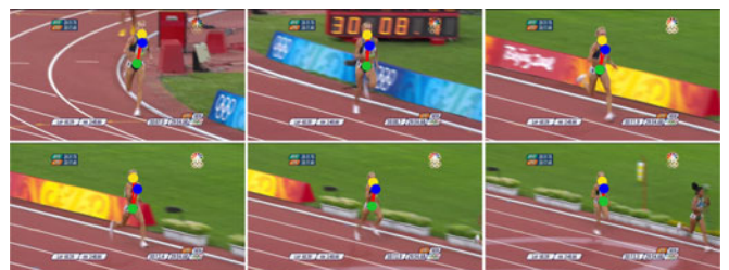
Fig. 14. Matching using edge pixels on a 400-frame sequence of a person running. The detection rate is 97 percent. Average running time is 0.7 s per frame.
