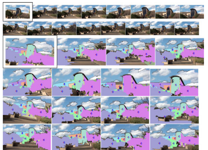
Fig. 18. Matching an outdoor scene using superpixels. The first images in rows 1 and 3 show the template image and the region template. Nine regions are found on the template and form a graph model. Using the template we match regions in the target images. Original target images are shown in rows 1-2. The matching results are shown in rows 3-6.
