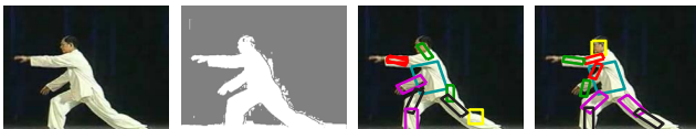
Fig. 5. Compare with pose estimation using max covering which ignores the consistency constraints. From left to right: Input image, foreground map, pose estimation using max covering, and the result of consistent max covering.
