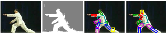
Figure 4. Compare with pose estimation using max-covering which ignores the consistency constraints. From left to right: input image, foreground map, pose estimation using max-covering and the result of consistent max-covering.
