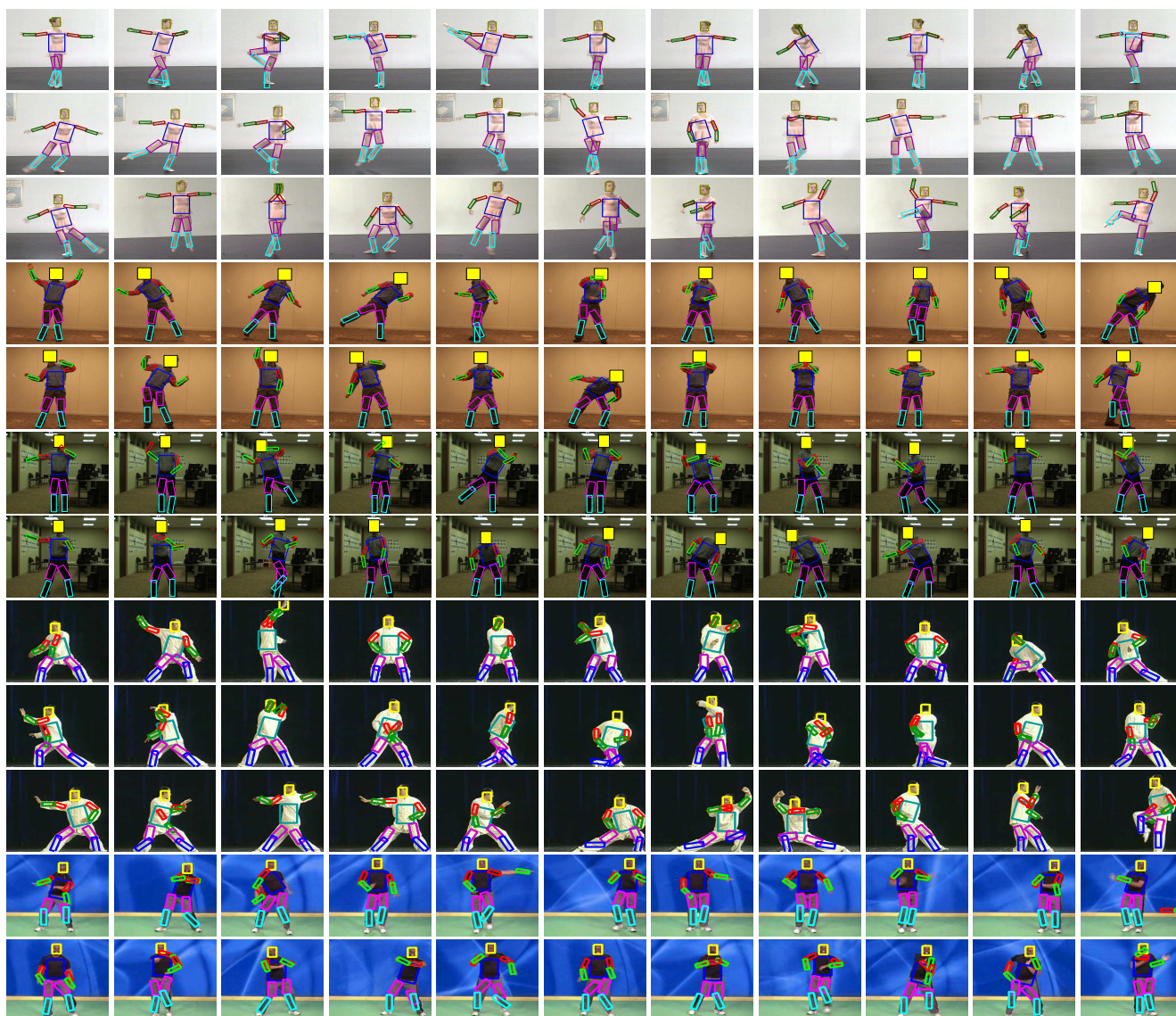
Figure 11. Pose estimation using consistent max-covering for the 6 test videos. Ballet has complex movements, self-occlusion, fast motion and interleaving effects; Lab involves baggy clothes, cluttered background and foreground; Actors wear baggy clothes in taichi and fitness sequences from YouTube. We use simple color segmentation to extract foreground maps for all the sequences except lab-II for which we use background subtraction. Row 1: sample results for 301-frame ballet-I; Rows 2-3: sample results for 314-frame ballet-II; Rows 4-5: sample results for 186-frame lab-I; Rows 6-7: sample results for 276-frame lab-II; Rows 8-10: sample results for 303-frame taichi; Row 11-12: sample results for 84-frame fitness.
